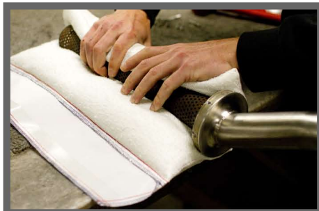
Step 6: With the exhaust shell removed, discard of the old packing and wrap the new packing around the core.
