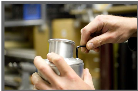
Step 5: Using a 4mm allen key, loosen the allen screws on the end cap.
