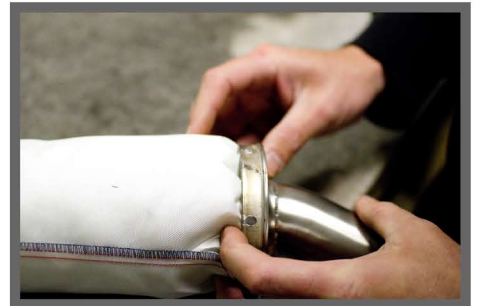
Step 8: Tuck the packing underneath the inlet.
