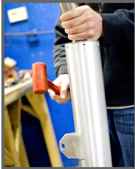
Step 4: Using a rubber mallet, tap the exhaust shell to remove the inlet.
