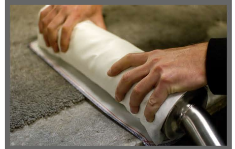
Step 7: When wrapping the packing around the core, make sure to make it as snug as possible.
