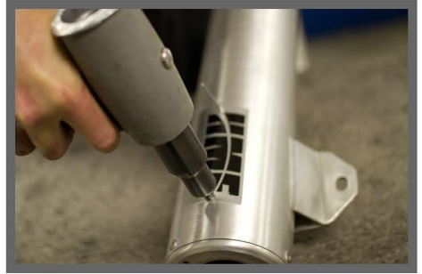
Step 16: Using an air rivet gun, secure the rivets to the exhaust shell.
