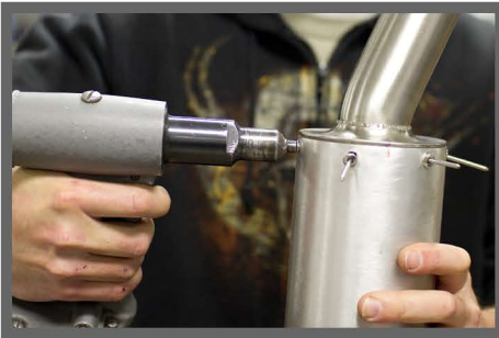
Step 14: Using an air rivet gun or automotive style riveter ( small hand riveter will not work ), secure all rivets on the inlet.
