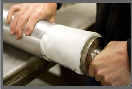
Step 10: Slide the core into the exhaust shell.
