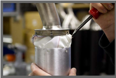
Step 11: Using a small screwdriver or pry bar, tuck the packing in the exhaust shell.
