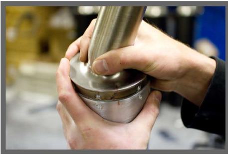
Step 12: Push the inlet completely into the exhaust shell, lining up the rivet holes and your marker mark. ( See step 13 )
