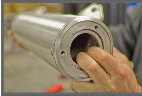
Step 13: You may need to pry the core sideways to catch the end cap lip.
